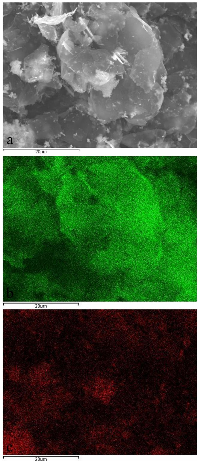
**Fig. 5.** Elemental composition of for the lowest ZnO nanopowder concentration: (a) SEM image, (b) distribution of C (green color presenting C), (c) distribution of Zn (red color presenting Zn). (For interpretation of the references to color in this figure legend, the reader is referred to the web version of this article.)
