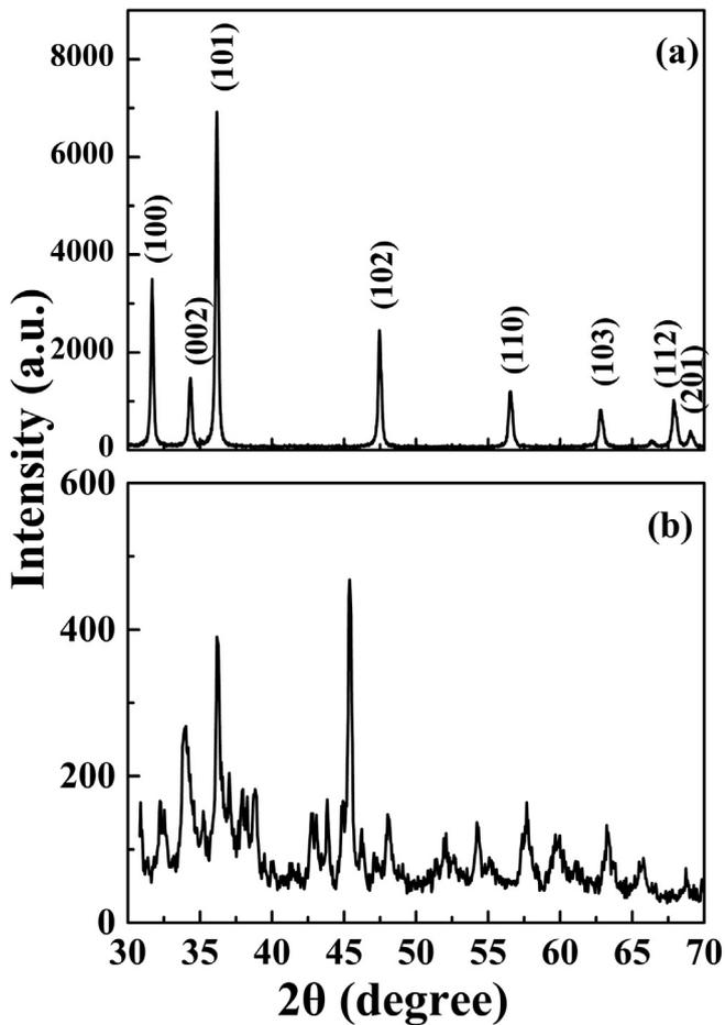
Fig. 2. XRD patterns of: (a) ZnO nanopowder grown using zinc acetate with 2-propanol:H<sub>2</sub>O and (b) ZnO nanopowder grown with pure water.
