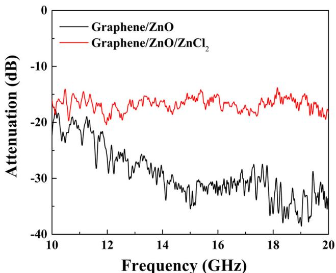
Fig. 3. Electromagnetic interference shielding of nanocomposite layers based on (a) ZnO nanopowder and graphene nanoplatelets and (b) ZnO nanopowder, graphene nanoplatelets and ZnCl<sub>2</sub>, both having a ZnO nanopowder/graphene nanoplatelets ratio of 1.5.
