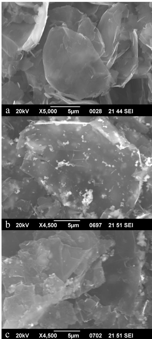
**Fig. 4.** SEM images of: (a) the commercial graphene flakes, (b) the composite with the lowest ZnO nanopowder/graphene nanoplatelets ratio and (c) the composite with the highest ZnO nanopowder/graphene nanoplatelets.
