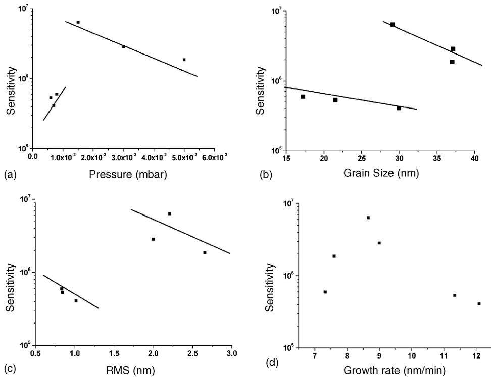
Fig. 6. Sensitivity correlations for InO<sub>x</sub> films grown at different pressures: (a) sensitivity vs. pressure, (b) sensitivity vs. grain radius, (c) sensitivity vs. RMS and (d) sensitivity vs. growth rate.
