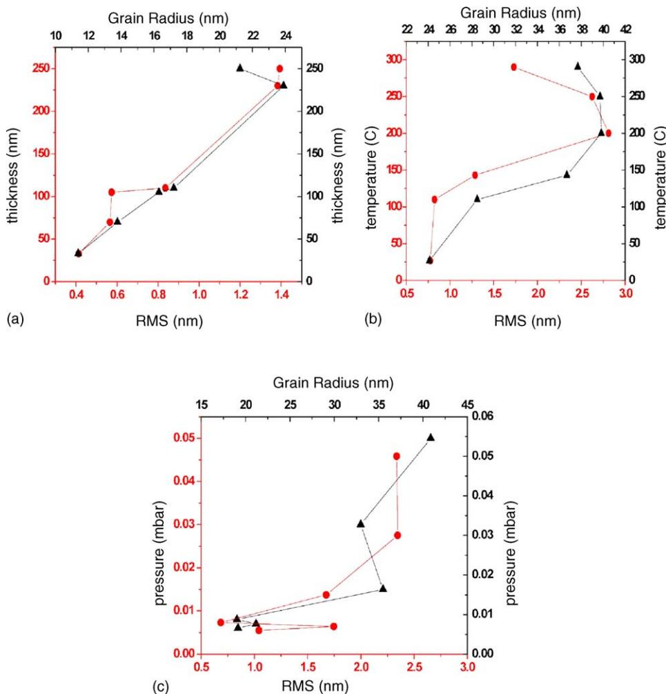
Fig. 2. (a) RMS (●) and grain size (▲) from AFM measurements as a function of film thickness. (b) RMS (●) and grain size (▲) from AFM measurements as a function of deposition temperature. (c) RMS (●) and grain size (▲) from AFM measurements as a function of deposition total pressure.
