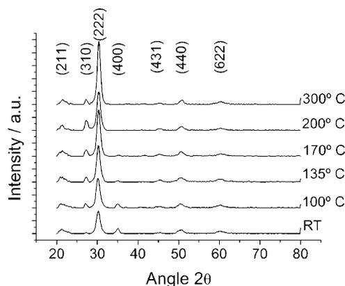
Fig. 3. X-ray diffractograms of InO<sub>x</sub> films prepared at different substrate temperatures.
