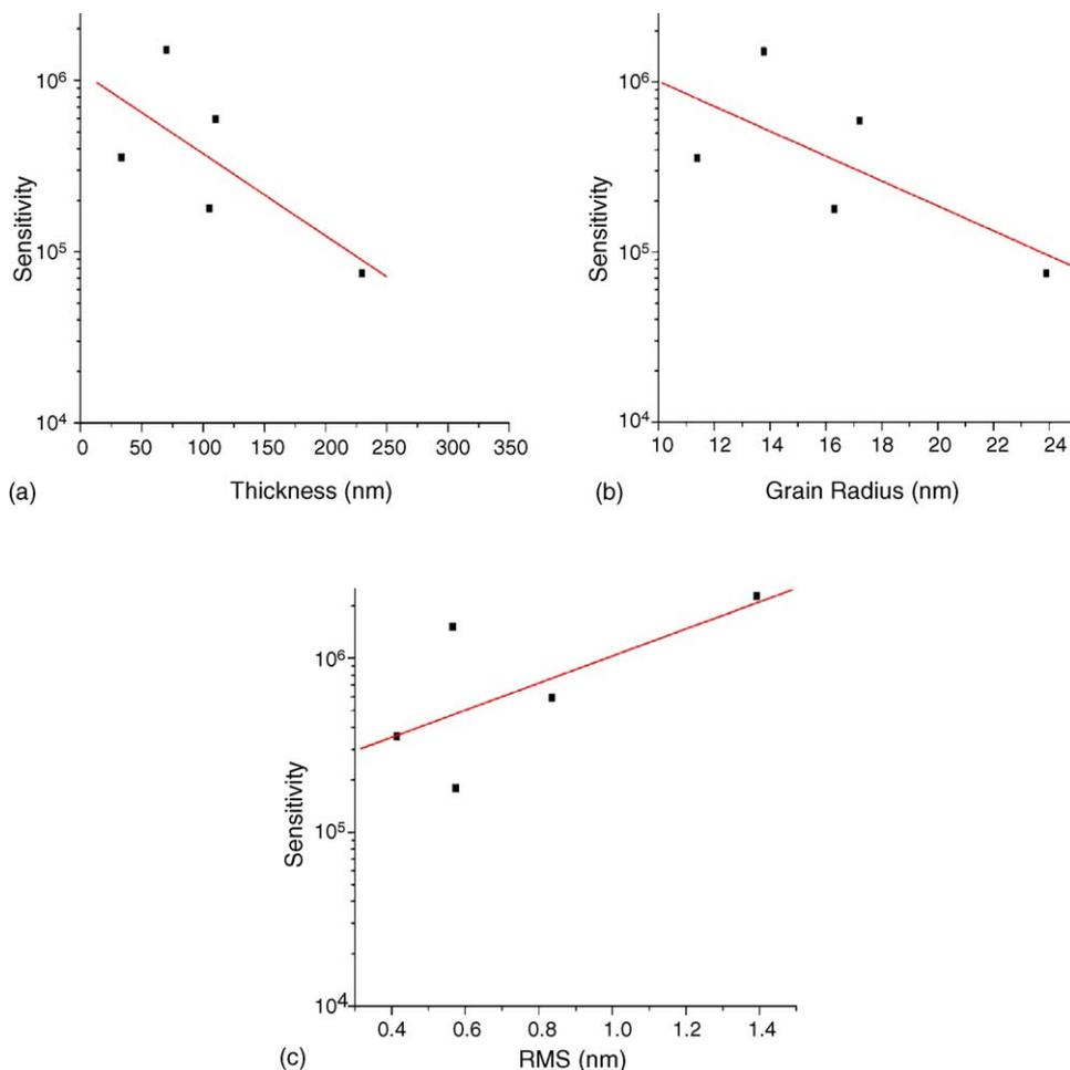
Fig. 4. Sensitivity correlations for the  $\text{InO}_x$  thickness series: (a) sensitivity vs. thickness, (b) sensitivity vs. grain radius and (c) sensitivity vs. RMS.
