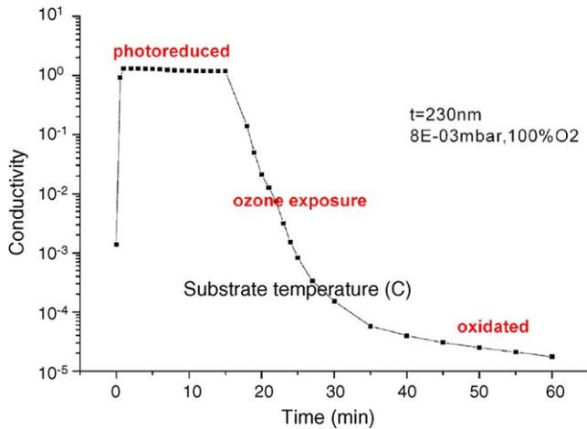
Fig. 7. Typical photoreduction–oxidation conductivity curve for  $\text{InO}_x$  thin films. The photoreduced state corresponds to maximum conductivity; the oxidized state corresponds to minimum conductivity.
