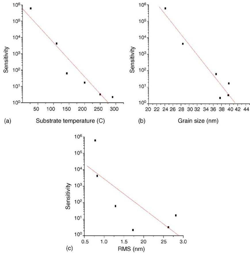
Fig. 5. Sensitivity correlations for InO<sub>x</sub> films grown at different substrate temperatures: (a) sensitivity vs. substrate temperature, (b) sensitivity vs. grain radius and (c) sensitivity vs. RMS.
