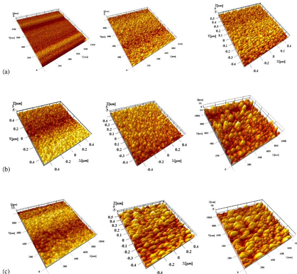
Fig. 1. (a) AFM images of  $\text{InO}_x$  films with different thickness  $t = 33, 110, 230 \text{ nm}$ . (b) AFM images of  $\text{InO}_x$  films grown at different substrate temperatures  $T = 27, 140, 200^\circ\text{C}$ . (c) AFM images of  $\text{InO}_x$  films grown at different total deposition pressures  $p = 6, 30, 50 \mu\text{bar}$ .
