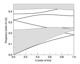
FIG. 6. Dispersion relation for the PC waveguide, with f = 60%. The gray area is the projected band structure of the perfect 2D crystal. The bold solid lines correspond to TE guided modes even with respect to the waveguide's axis.
