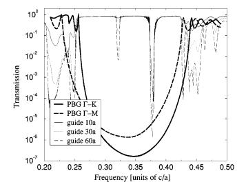
FIG. 2. Transmission spectra for various lengths of the waveguide, with f=60%. The bold solid (dotted) line delimits the  $\Gamma$ -K ( $\Gamma$ -M) PBG of the bulk PC. The solid, dotted, and dashed lines correspond to the transmission along the waveguide (source in position 1) with length 10*a*, 30*a*, and 60*a*, respectively.
