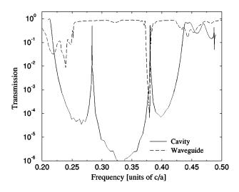
FIG. 5. Transmission spectra for the 1D cavity (solid line) and the waveguide (dotted line), with f = 60% and length 10*a*. For the 1D cavity it is intended that the transmission is calculated along the  $\hat{y}$  direction, with the source in position 2, see Fig. 1.
