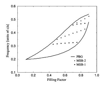
FIG. 3. Position of the MSBs vs f. MSB-1 (MSB-2) is for the type low-frequency (high-frequency) MSB of Fig. 2. The solid lines give the width of the TE gap for different f.
