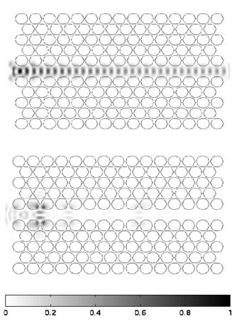
FIG. 4. Normalized intensity of the electric field for the frequencies corresponding to the (top panel) low-frequency MSB and (bottom panel) high-frequency MSB of Fig. 2.
