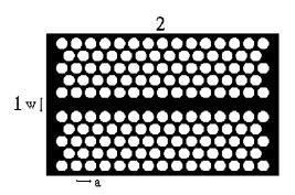
FIG. 1. Triangular lattice of air holes in GaAs ( $\epsilon = 11.56$ ). The missing holes yield a waveguide of width *w* along the  $\Gamma - K$  direction; *a* is the lattice constant; 1 and 2 mark the positions of the source.
