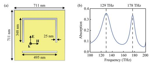
Fig. 1. (a) Unit cell of the complementary SRR metamaterial. (b) Absorption spectrum of the same metamaterial.
