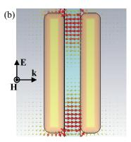
Fig. 5. (a) Unit cell of the wire-pair metamaterial. (b) Electric field at the resonance frequency of the magnetic dipole mode. Note that the large resonant electric field is mostly perpendicular to the substrate.
