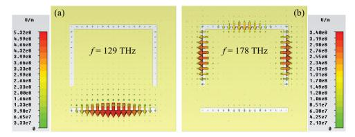
Fig. 2. (a) Electric field patterns of the resonances of the complementary SRR metamaterial shown in Fig. 1 (without graphene). (a) Fields concentrated in the slit at  $f=129\,\mathrm{THz}$ . (b) Fields concentrated in the U-shaped ring at  $f=178\,\mathrm{THz}$ .
