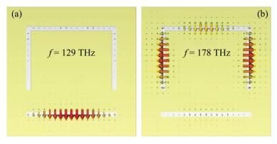
Fig. 4. Current density in the graphene sheet. The current density simply follows the resonant electric field of the resonances of the complementary SRR structure.
