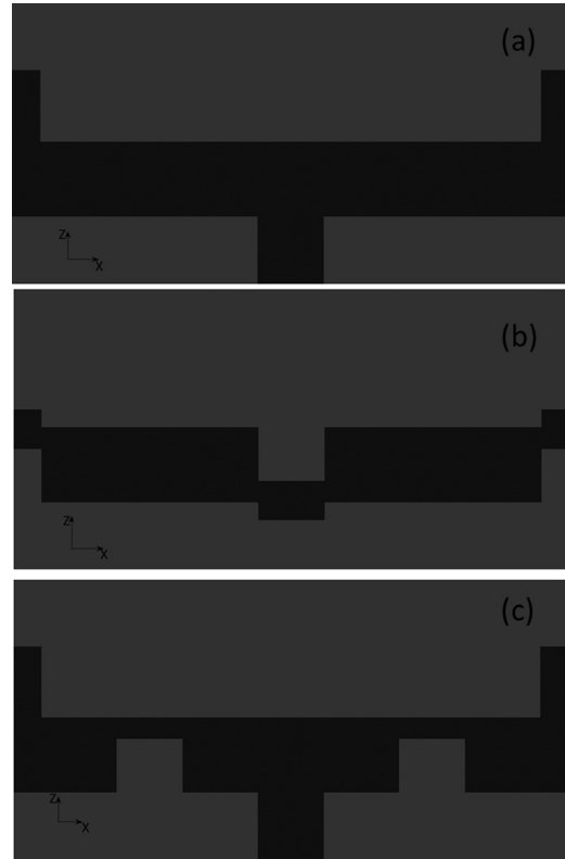
FIG. 5. Two proposed modified layer-by-layer structures. (a) A cross section of the x - z plane of the unmodified structure studied. (b) x - z plane of the Modified Structure 1 at the same y coordinate as in (a). Material is removed from each rod of all the layers from the parts of each rod that there is overlap with the rods from the above layer. (c) x - z plane of the Modified Structure 2 at the same y coordinate as in (a). Material is removed from each rod of all the layers from the parts of the rod that there is no overlap with the rods from the above layer. The same amount of material is removed from each rod in both cases.
