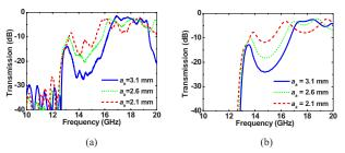
Fig. 7. (Color online) (a) Experimental and (b) simulated transmission spectra of fishnet structure for different sizes of the unit cells along propagation direction,  $a_k$ .
