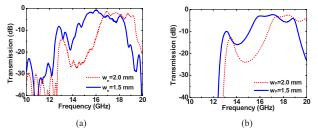
Fig. 2. (Color online) (a) Experimental and (b) simulated transmission spectra for fishnet structures with different width of necks. Solid lines,  $w_n = 1.5$  mm; dotted lines,  $w_n = 2$  mm.
