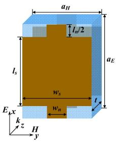
Fig. 1. (Color online) Schematic of the unit cell of the fishnet structure. **E**, **H**, and **k** correspond to electric field, magnetic field, and wave vector, respectively.  $a_E$  and  $a_H$  are the x and y size of unit cells, respectively.  $l_s$  is the length of the slabs,  $w_s$  the width of the slabs,  $w_n$  the width of the continuous wires (necks),  $l_n$  the length of the neck parts, and t the thickness of the dielectric substrate.
