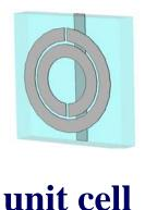
*Fig. 6.* The metallic double split ring resonator (SRR) combined with a continuous metallic wire (on the back side of a dielectric) make up the unit cell of a LHM.
