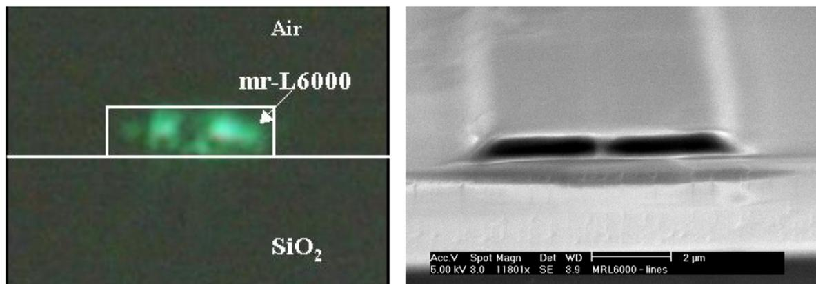
FIG. 4: Image of light guided in a mr-L 6000 slab polymer waveguide. White lines show the cross section of the polymer waveguide with dimension 1 μm × 6 μm (left). SEM cross-section image of the 1 μm wide strip written on a film of mr-L 6000 film-thickness on the line written sample. This is a typical mr-L 6000 waveguides written on silicon oxide substrate, by electron beam writing (right).
