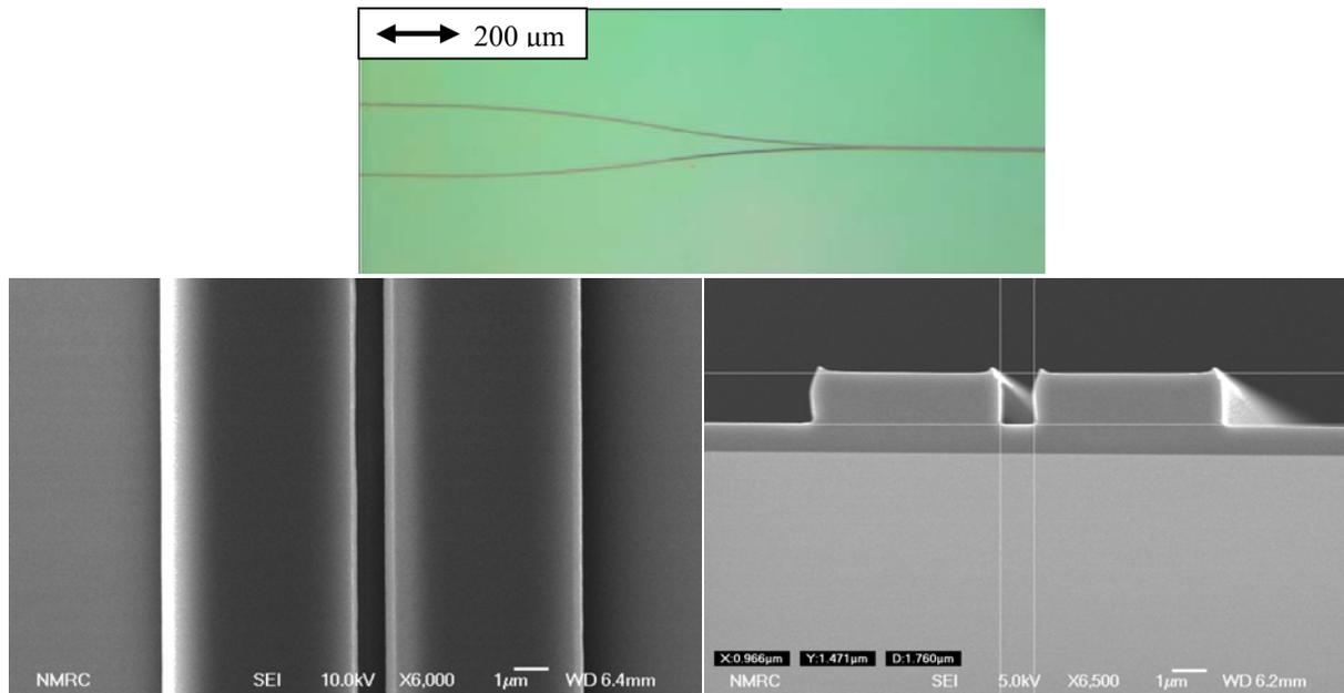
FIG. 3: Optical microscope image of a section of an interferometer (the two waveguides comes in near interaction, top) and SEM images of the two interfering waveguides (bottom).
