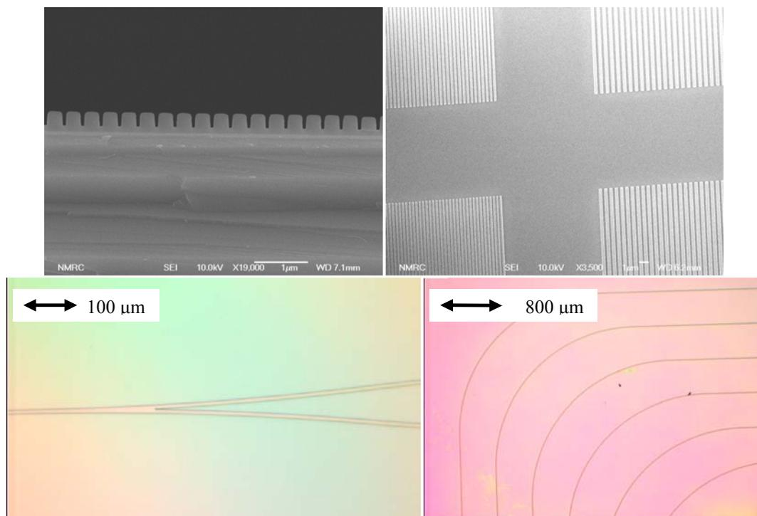
FIG. 2: SEM images of gratings imprinted in mr-L 6000 (top) and optical microscope image of a section of an interferometer (splitter, bottom left) and of bended waveguides (bottom right) imprinted in mr-L6000.
