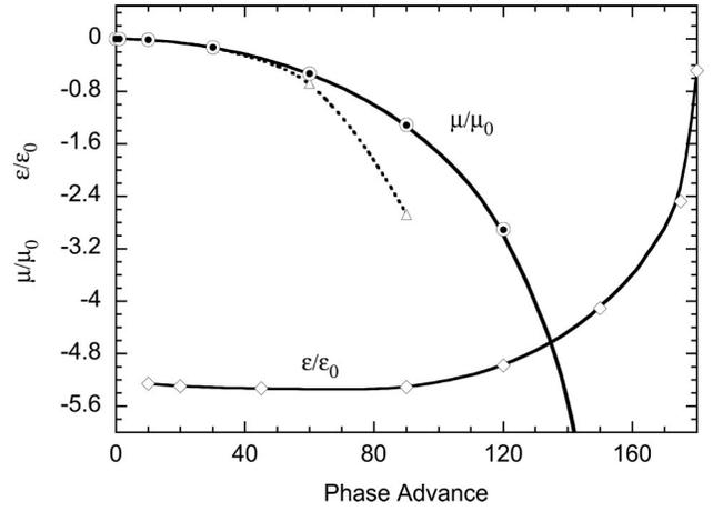
FIG. 3. Calculated permeability (open and closed circles, triangles) and permittivity (diamonds) for the left-handed propagation band of the composite SRR-wire structure. Open circles:  $\langle B \rangle / \langle H \rangle$  method; closed circles:  $z, n$  method; triangles: currents method. The permittivity was calculated by the  $z, n$  method only.
