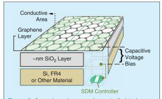
Figure 5. A graphene layer can be controlled to become transparent to electromagnetic waves locally, enabling the formation of MM patterns upon them. The SDM controllers form an array of local capacitors with the continuous  $SiO_2$  and graphene layers by regulating their voltage [12].
