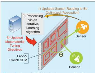
**Figure 8.** A potential SDM application scenario, featuring an angle-independent electromagnetic absorber, accentuating the SDM programmability, interconnectivity, and adaptivity potential.
