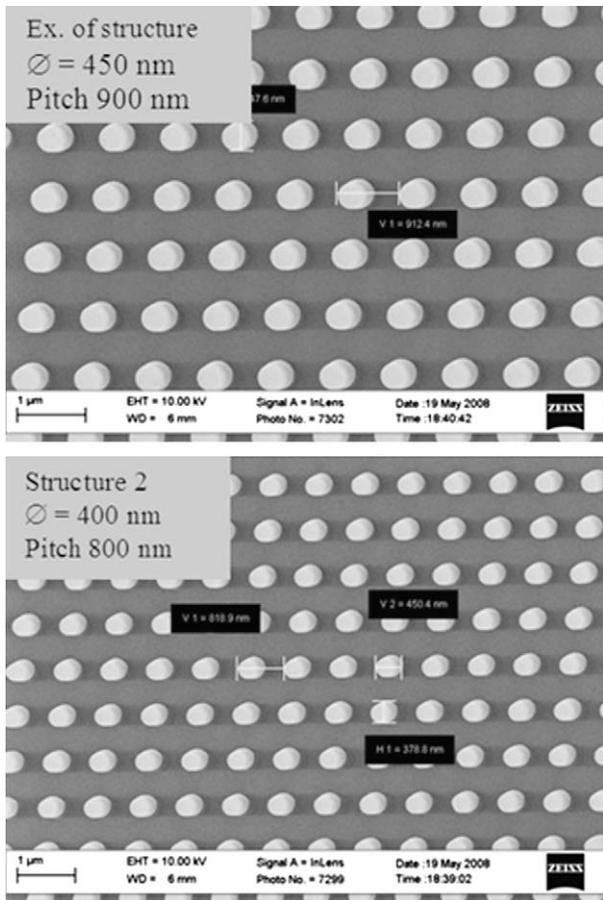
Fig. 1. SEM images of nanoimprinted metallic structures with their associated critical dimension.
