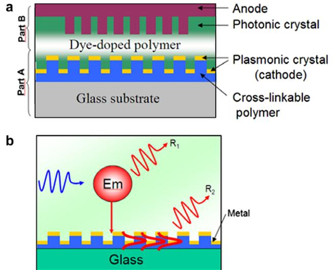
Fig. 2. (a) Cross-section schematic of the system. Part A shows the studied system in this manuscript. Part B presents the next fabrication step for potential OLEDs application and (b) schematic of the alternative recombination path (named  $R_2$ ) to the conventional radiative recombination (named  $R_1$ ) in the near field of the metal layer in order to enhance light extraction.
